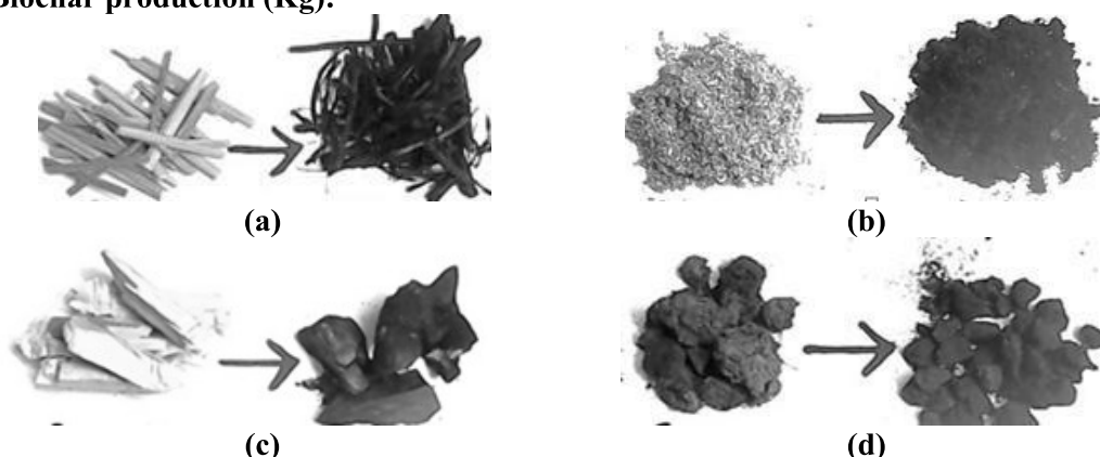
Figure 1. Biochar produced from four different feed stocks namely (a) Rice straw, (b) Saw dust, (c) Wood and (d) Cow dung.
